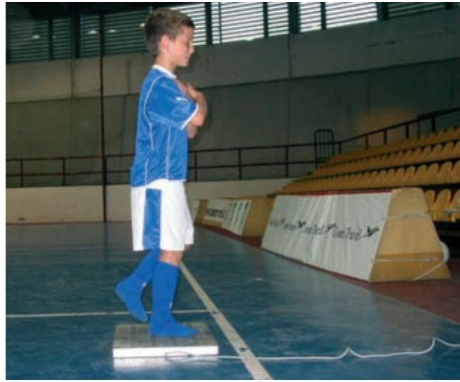
"BALANCING TEST CARRIED OUT BY FORCE MEASUREMENT PLATFORM CONNECTED TO SERVICE LAB BOSCO SYSTEM"
